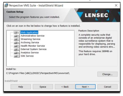
**PVMS Web Application**: The application server component of Perspective VMS. The Web application is responsible for generating the Graphical User Interface (GUI).
