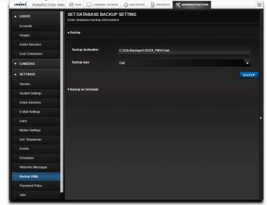
3. Expand 'Backup' (1) to reveal the backup destination field (2). You can list a folder in any location that is accessible from this server. You will name the backup destination file. If the folder has not been created yet, Perspective VMS will create it.
