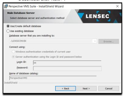
NOTE: The Database Server instance name and password will need to match the instance name provided by the customer or created when installing SQL.
