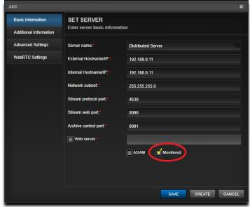
2) Now that you have the distributed server set up in PVMS on the primary server, you can now begin the installation of PVMS on the distributed server. **NOTE: if you are adding a distributed server to an already existing network, it is very important that you back up the SQL database on the primary server BEFORE starting the distributed server PVMS installation.**
