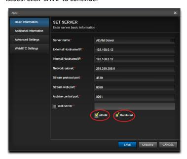
2) Now that you have the Distributed-ADAM Server set up in PVMS on the primary server, you can now begin the installation of PVMS on the distributed server. **NOTE: if you are adding a distributed server to an already existing network, it is very important that you back up the SQL database on the primary server BEFORE starting the distributed server PVMS installation.**
